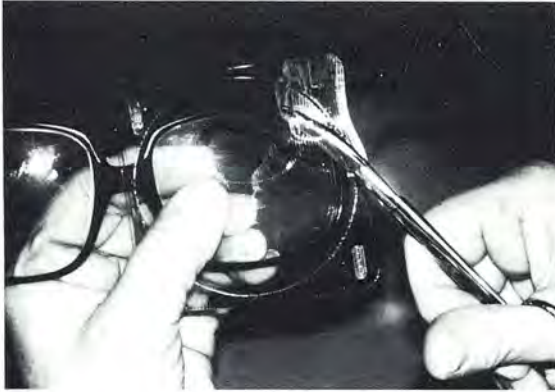
Figure 2. Prism is cut on outside of lens, 1/2 mm inside of frame.
